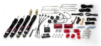
●The damping force can be easily adjusted from a controller inside your vehicle (Choose from 96/64/32 levels of adjustment). By utilizing a stepping motor, a maximum of 96 levels of adjustment is possible to finely tune the vehicle setup for your desired ride quality.
