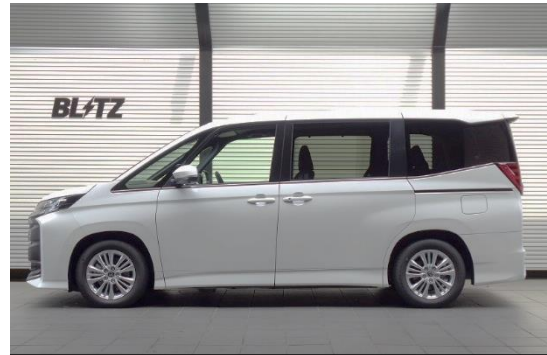
Front : 28mm Down / Rear : 59mm Down
