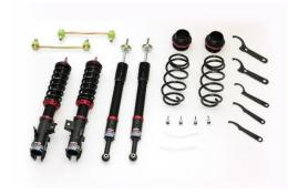
■ Remarks: 2WD. Rear adjustment dials can be installed without any modifications,
