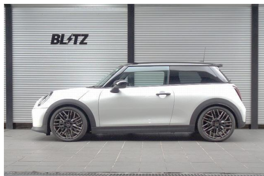
Front : 28mm Down / Rear : 21mm Down
