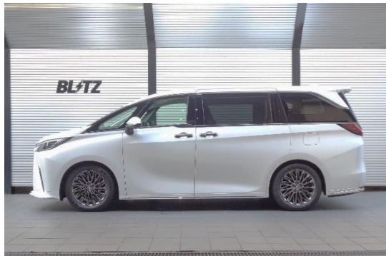
Front : 16mm Down / Rear : 26mm Down
